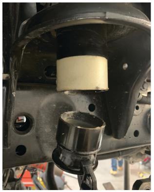
Fig. 2a: Cut the bump holder off under the tape line. Passenger side shown.
