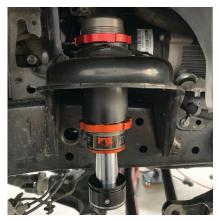
Fig. 5: Install the lock rings.
