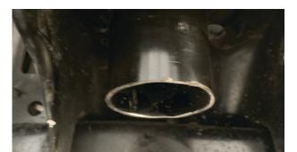
Fig. 3: Cut the bump holder off under the tape line. Passenger side shown.
